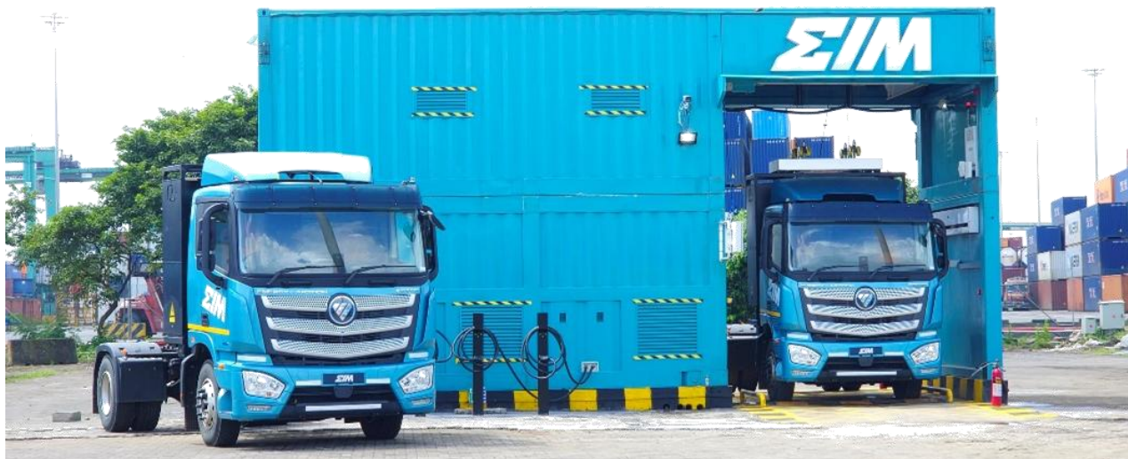
EIM's heavy commercial vehicle swap-and-charge hub, with Ashwa electric tractor-trailers at a battery swapping station. Under the HPCL agreement, hubs of this type will be deployed at retail outlets along major freight corridors.
